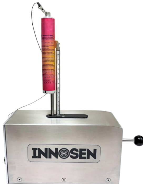
Image 8: The Tube Probe IS9561 with a sample aluminium collapsible tube
