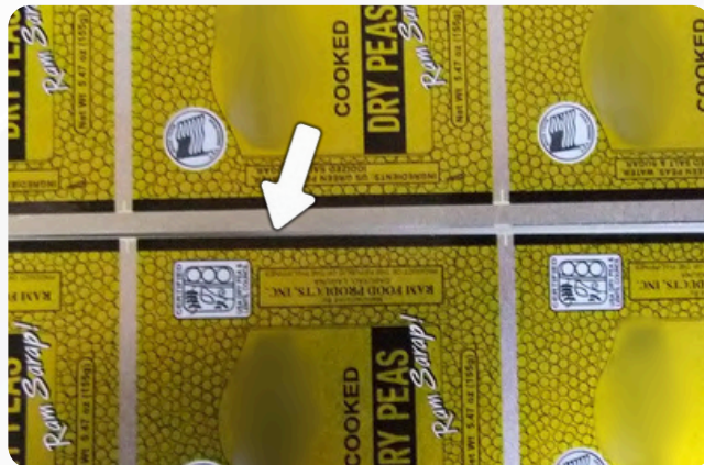
📷: Sheet moved sideways. Lacquer or print is on the margin.
