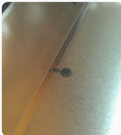
📷: Grease/Tar droplet on the margin
